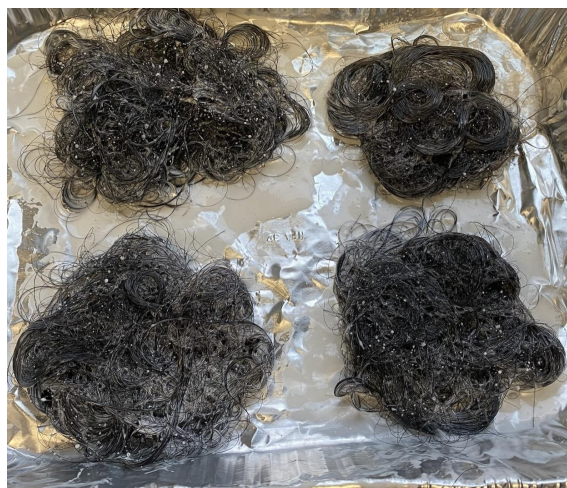
Figure 1. Human hair engineered into a composite material and pressed into mats.
