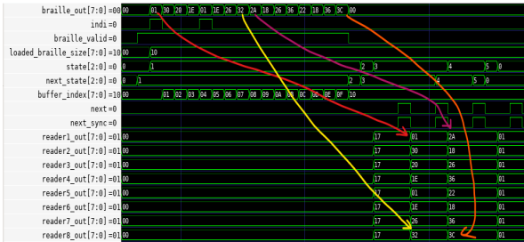
Figure 14. Simulation waveforms of Braille Buffer/Reader
